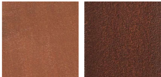
oxidised corten steel waxed oxidised corten steel
